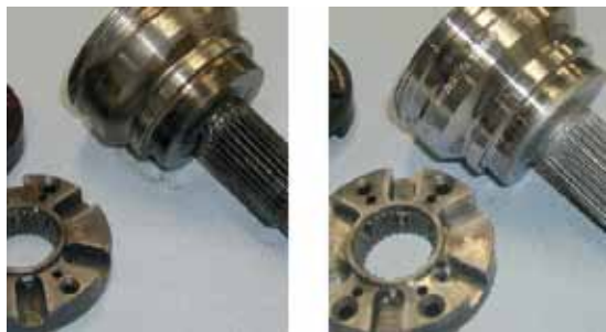
Removal of oxidation and other contaminants
